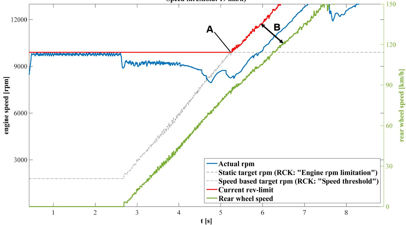
Figure 34 Rev-limiter during Launch-Control
