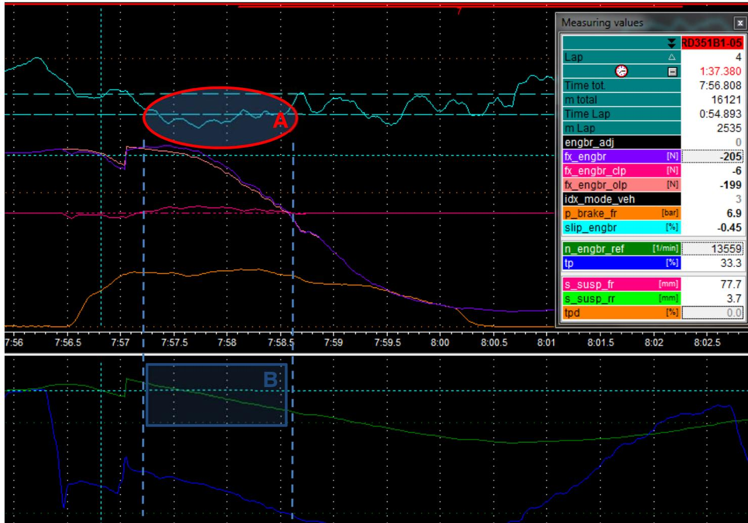
Figure 42 Example intervention of the closed loop controller
