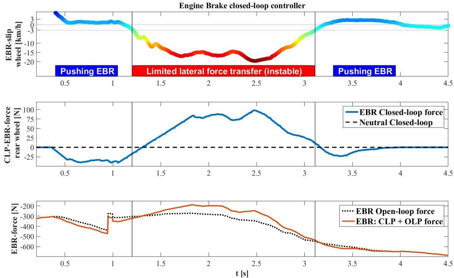
Figure 17 "Engine brake closed-loop controller"
