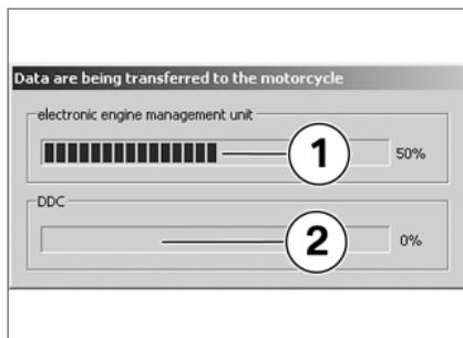
The progress bar **1** indicates the current transfer status. The transfer may take a few seconds. If the DDC is installed, the data for the DDC is transferred in addition to the data for the engine control unit. An additional progress bar **2** appears.
