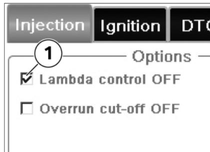
The lambda control system analyses the signals from the oxygen sensors fitted as standard in the exhaust system and corrects fuel injection timing in order to achieve a stoichiometric fuel/air ratio for combustion. If tick **1** is not set in the as-delivered condition, this only means that the as-delivered condition shall not be changed (lambda control is not necessarily active). Whether or not lambda control is active depends on the exhaust system
