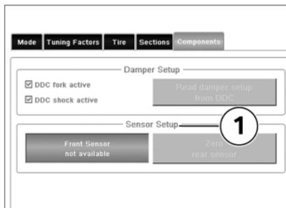
Front forks and/or spring strut can be deactivated under Damper Setup. In the standard configuration (RCK not active) riding with only one of the two DDC components is not possible, as in this case the component still being installed is not activated anymore for safety reasons. For example, if the front forks must be replaced with a conventional part after a crash, it can be deactivated as DDC component. Spring
