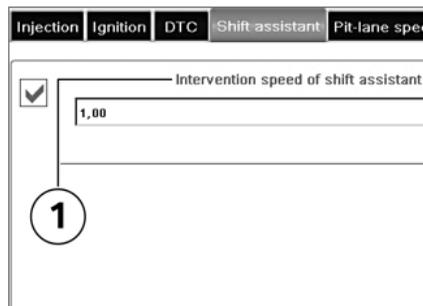
The shift assistant allows upshifting of the gearbox without operating the clutch. While the engine torque reduction for initiating upshift using the shift assistant cannot be changed, the way in which engine torque is built up after the upshift can be influenced by changing the applicable factor "Intervention speed of shift assistant" **1**. Values greater than 1 mean that torque is built up more quickly, values less than 1 slow down the build-up of engine torque. A value of 1 means that
