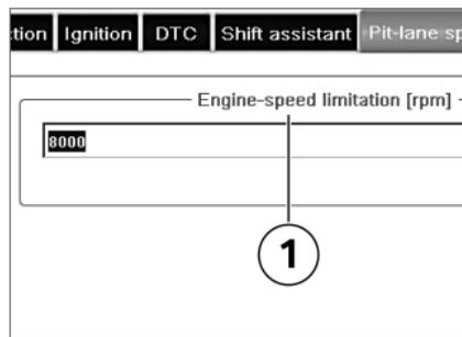
This function enables the use of an rpm limiter that is active only in 1st gear and only when the starter button is pressed. Engine speed limiting **1** can be adjusted so that, for example, the motorcycle cannot be accelerated
