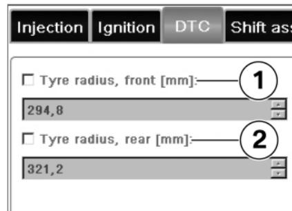
In order to correctly compute the wheel speed, the radii of the front and rear tyres for straight-ahead driving have to be entered (front tyre radius **1** and rear tyre radius **2**).
