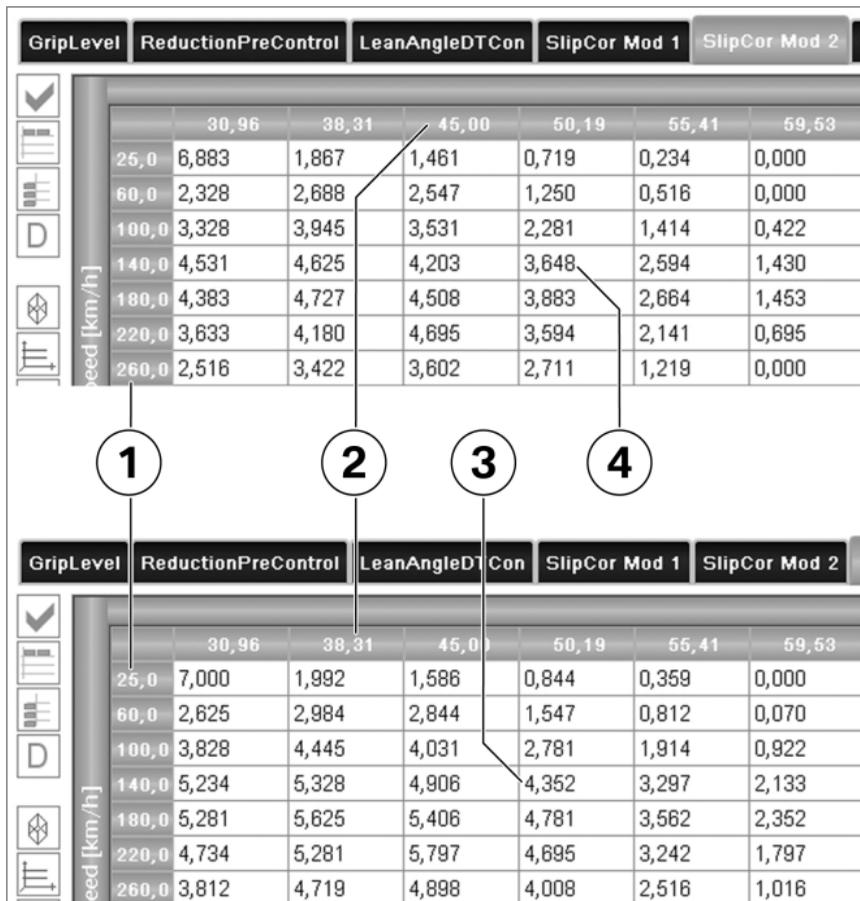
In the characteristic map the speed **1** is indicated in km/h and the heel angle **2** in degree.
