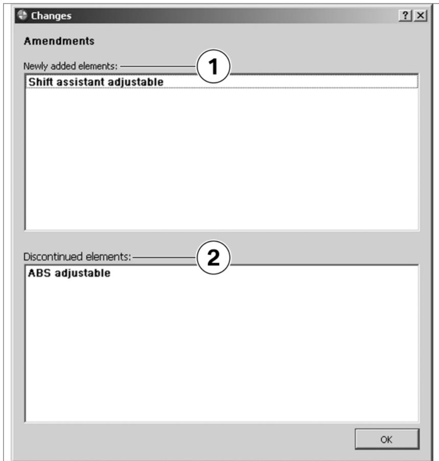
In the case of retrofits (e.g. of a shift assistant) the changed configuration is automatically detected and displayed in the BMW HP Race Calibration Kit. Added elements **1** enable the respective tab in the working area allowing them to be edited. Omitted elements **2** deactivate the respective tab in the working area. They cannot be further edited.
