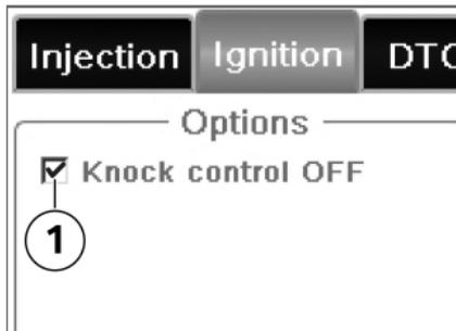
You can deactivate knock control by ticking the box in front of **1**. Knock control analyses the signals from the knock sensors and corrects the ignition timing to avoid knocking engine operation in the combustion process (see below). It can be deactivated in order to suppress interventions in the ignition timing output. Knock control intervenes only in circumstances in which knocking combustion occurs, however, so it is advisable not to deactivate it.
